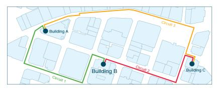
A basic FibreLINK ring network will significantly increase your network reliability. The example shown above is made up of three FibreLINK circuits making a ring between three buildings. This arrangement will ensure that a single fibre failure will generally not adversely affect any site on the network. However a major equipment failure or fibre cut to the single cable entry into the building could isolate one site – leaving the two remaining sites unaffected.
