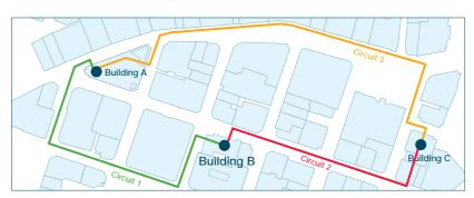
Even greater network reliability can be achieved by engineering two completely diverse cable entries into a building (i.e. on the East and West side of the building) and then deploying duplicated networking equipment (i.e. in the East and West facing directions). This arrangement will ensure that a single equipment failure or fibre cable cut will not isolate any site on the ring. CityLink's engineering team will work with you to achieve appropriately diverse cable entry into your sites.
